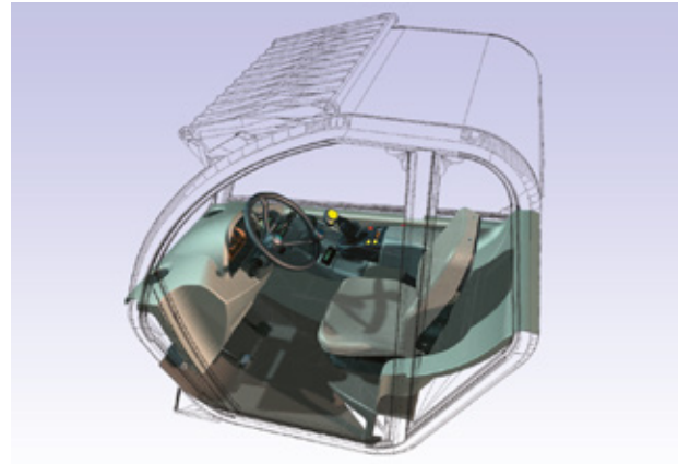
Interni cabine per macchine movimento terra Interior cabin trim for construction machinery
